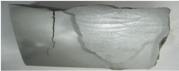
Fig.9: Micrograph showing welded joints and crack in the base metal
