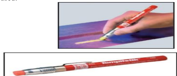
Fig.7. Temperature sensitive crayons (courtesy: TWI)
